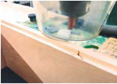
▲ Pic.29 Then I cut the rebate for the back panel and the rebate for the centre mirror. For the back panel rebate I used the overhead router...
